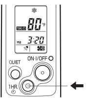
This function causes the unit to operate for one hour and then stop, regardless of whether the unit is on or off when this button is pressed.
